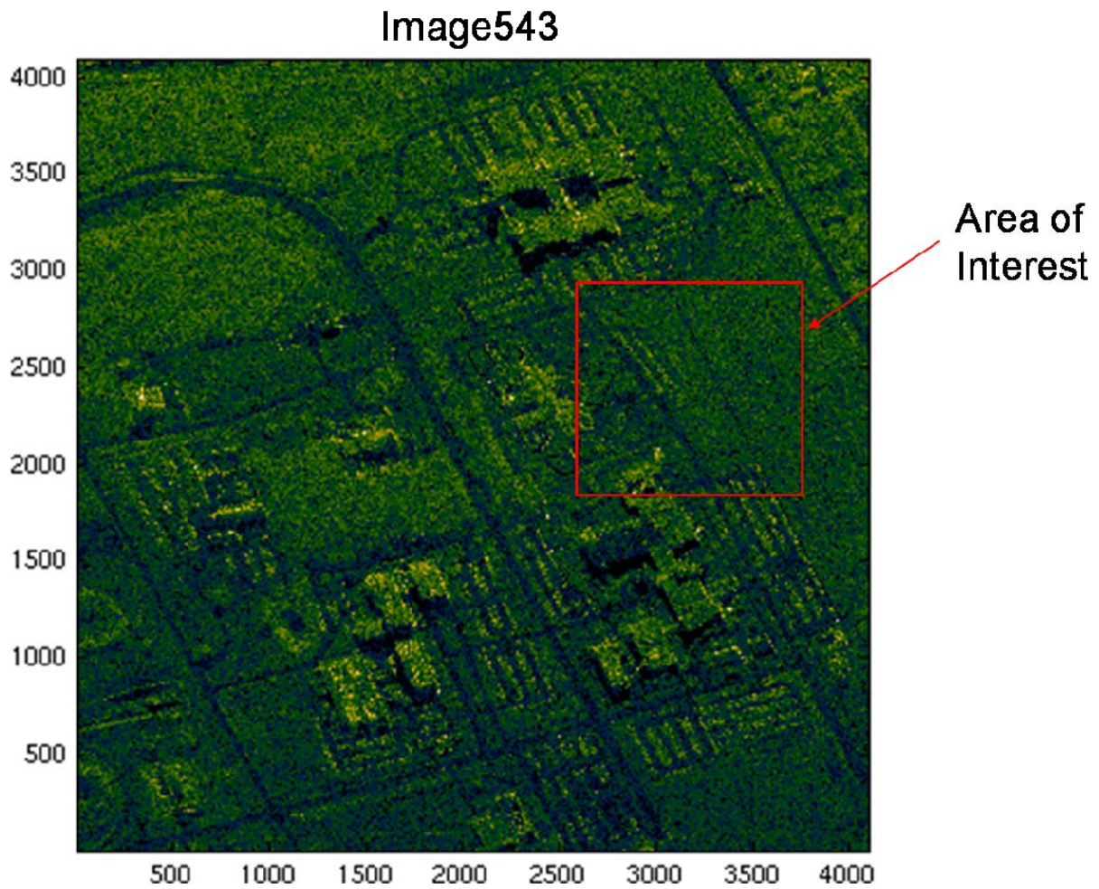
FIGURE 1: SAR REFERENCE IMAGE, SIZE = 4096 x 4096 PIXELS; AREA OF INTEREST, SIZE = 1024 x 1024 PIXELS.
